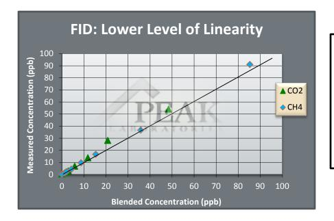
Figures 1 & 2 illustrate the lower detection limits of a FID analyzer monitoring compounds within Nitrous Oxide gas. Using Peak's pioneered hybrid platform results are delivered accurately while maintaining linearity, down to lower and upper levels.
