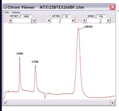
Benzene based chromatograph within Air, Inert or Oxygen matrix gases.
